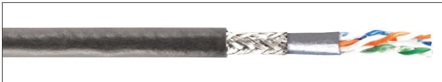
TRANSIT, 4 PAIR/24 AWG, SHIELDED FOIL TWISTED PAIR (SFTP) CAT 5, LOW SMOKE
